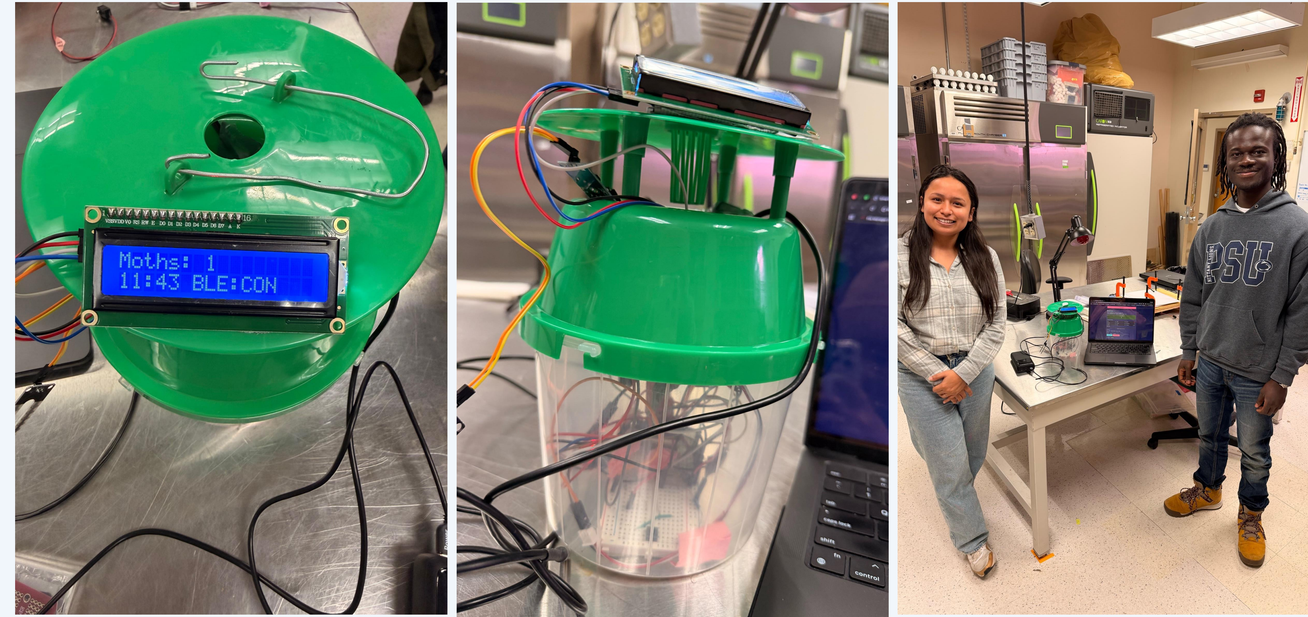
Fig 2. Automated trap structure, along with the assembled version in lab
